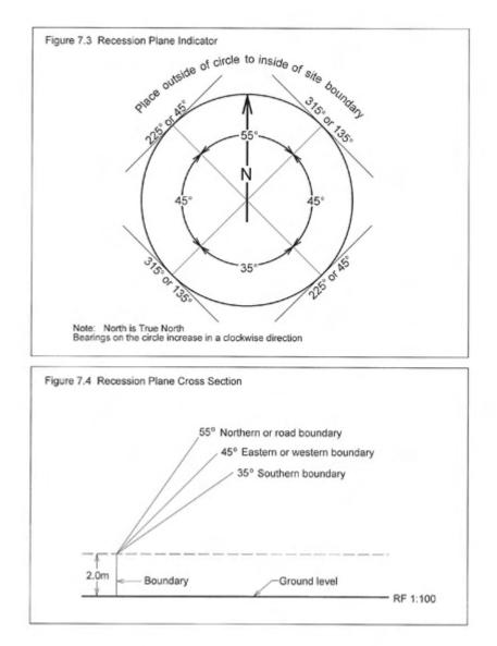
Diagram 7.3 - Recession Plane Indicator and Diagram 7.4 - Recession Plane Cross Section
